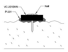
Apply a bead of P-201 before placing MC-2010MN on rough concrete. Apply sufficient P-201 to fill all voids or rough areas.
