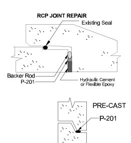
P-201 can be used in pre-cast applications such as utility vaults and storage reservoirs.
