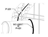
Apply a 1/4" by 1/2" bead of P-201 to the center of the existing wall. Remove any dirt or loose debris before applying the bead.
