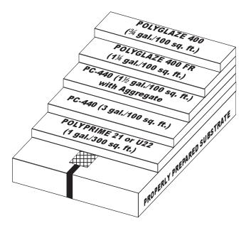
**Phase 2:** Prime concrete surfaces with Polyprime 21 or U22 at a rate of 1 gallon (mixture of Part-A & Part-B)/300 sq. ft. (0.14 liters/m²). Apply using a brush, airless sprayer or phenolic core roller. This will result in 3 dry mils (76 microns) of coating. Allow Polyprime to become tack free before proceeding to Phase 3.
